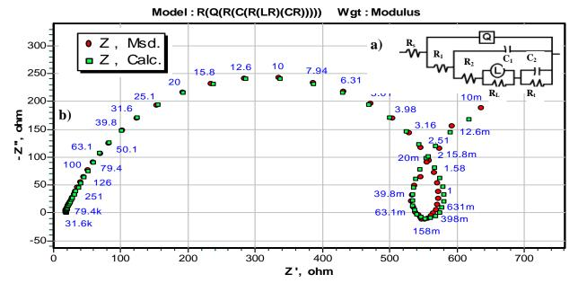
Figure 3b. Equivalent circuit model used to fit the experimental data of the base alloy.
