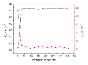
Figure 8. Dependence of  $R_P$  and  $C_{dl}$  on the immersion time for the corrosion of Al composite in 0.5M sulfuric acid solution.
