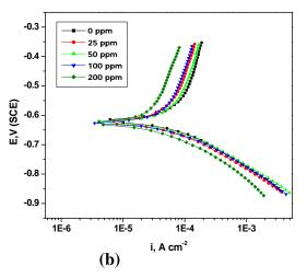
Figure 1. Potentiodynamic polarization curves for the corrosion of a) composite and b) base alloy in the presence of different concentrations of DEABT in 0.5 Msulfuric acid at 30°
