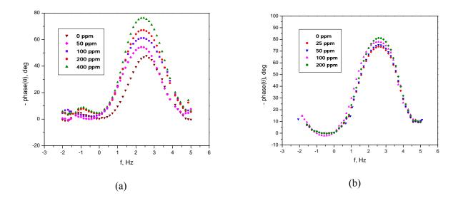
**Figure 4.** Bode plots for the corrosion of a) composite and b) base alloy in 0.5 M sulfuric acid at 30 °C in the presence of different concentrations of DEABT.
