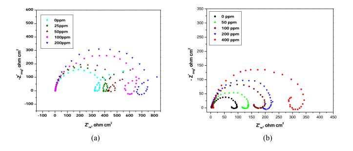
**Figure 2.** Nyquist plots for the corrosion of 6061 Al-SiC (a) composite (b) base alloy in 0.5 M sulfuric acid at 30 °C in the presence of different concentrations of DEABT.
