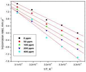
Figure 5. Arrhenius plots for the corrosion of composite in 0.5 M  $H_2$  SO<sub>4</sub> at 30 °C in presence of different concentrations of DEABT.
