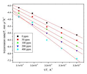
Figure 6. Plots of ln(corrosion rate)/T vs 1/Tfor the composite in 0.5 M H<sub>2</sub>SO<sub>4</sub> at 30 °C in the presence of different concentrations of DEABT.
