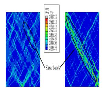
Figure 10: Local strain distribution in the DP microstructure with (a) MPF of 25% (b) MPF of 60% at uniaxial tensile strain of 10%.
