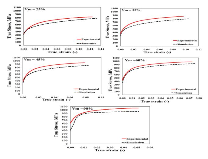
Figure 8: Comparisons between experimental and numerical flow curves of the investigated DP steels with varying martensite contents.
