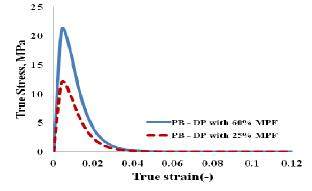
Figure 5 : Stress - strain curves representing phase boundary hardening for DP steels with 25% and 60% martensite.
