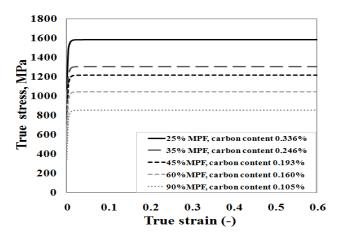
**Figure 7:** Modeled flow curves of martensite in the investigated DP steels having different MPF values and carbon content.
