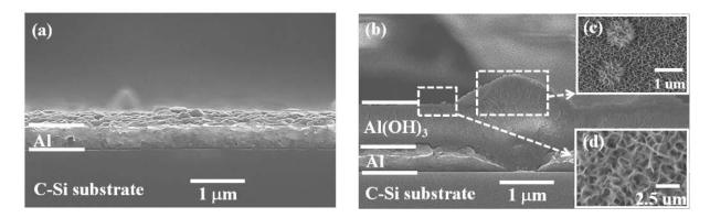
**Figure 1.** Top-viewed and cross-section FE-SEM micrographs: (a) the cross-section of as-deposited Al thin film before the alkaline treatment, (b) the cross-section of Al thin film after the alkali treatment, (c) the top-viewed of Al(OH)<sub>3</sub> after the alkali treatment and (d) the top-viewed of Al surface after the alkali treatment.
