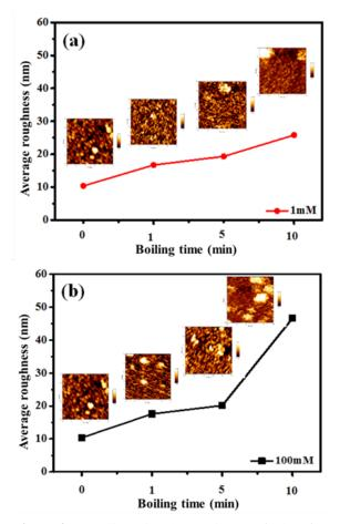
**Figure 3.** Two dimentional AFM image of Al surface after alikaline treatment with various boiling times at different KOH concentrations (a) 1 mM (b) 100 mM.
