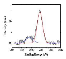
**Figure 5.** The XPS spectra of PTFE film deposited on Al treatment in KOH solution: C-C bonding in red line and –CF bonding in blue line.
