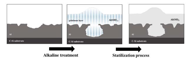
Figure 2. Mechanism forming Al(OH)<sub>3</sub> layer above the Al thin film by alkaline treatment process.
