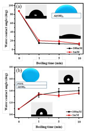
**Figure 4.** The contact angle measurement of (a)  $Al(OH)_3$  surface and (b) PTFE deposited on Al surface with various boiling time.
