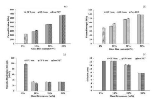
**Figure 3.** (a) flexural modulus (b) flexural strength (c) deflection and (d) impact strength of PBT and PBT/glass fiber composites.
