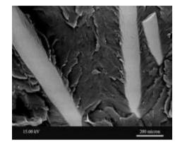
**Figure 2.** SEM micrographs of the fracture surface of PBT/glass fiber composites (mag. 500 x).
