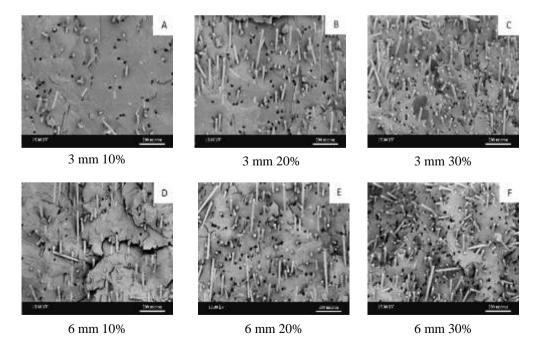
Figure 4. SEM micrographs of the fracture surface of PBT/glass fiber composites (mag. 50 x).
