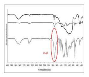
**Figure 1.** FTIR spectra: (A) Silane on GF, (B) PBT, and (C) PBT/GF Composite.
