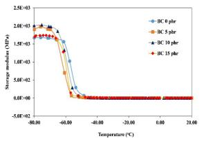
Figure 8. Storage modulus of NRL filled with BC composites.
