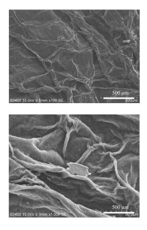
Figure 3. SEM micrographs of BC sheets.
