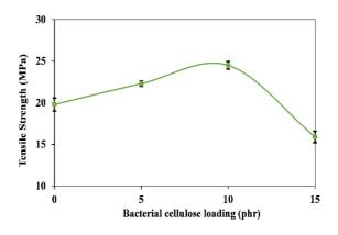
Figure 4. Tensile strength of NRL filled with BC composites.
