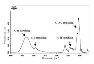
Figure 1. FTIR spectra of bacterial cellulose (BC).
