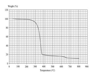
Figure 2. TGA thermogram of BC.
