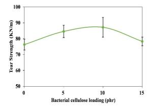
**Figure 7**. Tear strength of NRL filled with BC composites.
