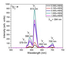
**Figure 5.** Emission spectra of KBSi:Eu<sup>3+</sup> glasses in the range of 500 to 750 nm.
