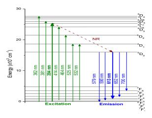
**Figure 7.** Energy level diagrams of Eu<sup>3+</sup> doped KBSi glasses.
