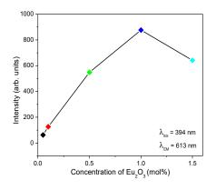
**Figure 6.** Relationship between the intensity of emission at 613 nm wavelength by excited 394 nm with the concentration of  $Eu_2O_3$ .
