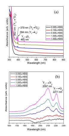
**Figure 3.** The Absorption spectra of the KBSi:Eu<sup>3+</sup> glasses.
