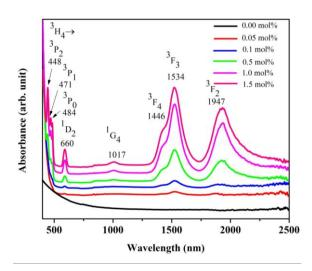
**Figure 4.** UV-Vis-NIR spectra of ZTB doped with  $Pr_2O_3$  concentration.
