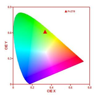
**Figure 8.** Color coordinates in the CIE 1931 chromaticity diagrams for 0.1 mol% of  $Pr_2O_3$  doped ZTB glasses under 448 nm laser excitation.
