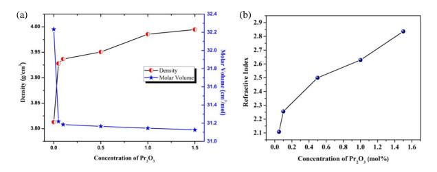
Figure 1. (a) Density, molar volume vs Pr<sub>2</sub>O<sub>3</sub> concentration and (b) refractive index vs Pr<sub>2</sub>O<sub>3</sub> concentration.
