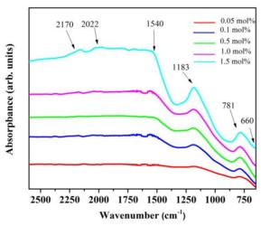
Figure 3. FTIR of ZTB doped with Pr<sub>2</sub>O<sub>3</sub> concentration.
