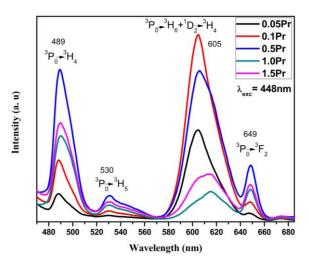
**Figure 5.** Emission spectra of ZTB doped  $Pr_2O_3$  concentration.
