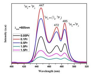
**Figure 6.** Excitation spectra of ZTB doped  $Pr_2O_3$  concentration.
