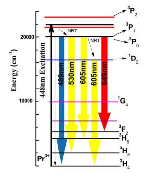
**Figure 7.** Energy level diagram of ZTB doped Pr<sub>2</sub>O<sub>3</sub> concentration.
