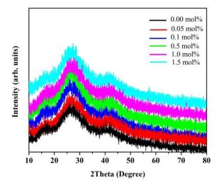
Figure 2. XRD of ZTB doped with Pr<sub>2</sub>O<sub>3</sub> concentration.
