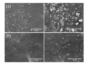
**Figure 3.** SEM micrographs with low (left) and high (right) magnifications of fracture surface of the selected rubber composites with various LCNO contents of (a) 1 phr and (b) 3 phr.
