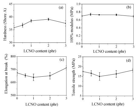
**Figure 5.** Mechanical properties of LCNO/ENR-25 composites with various LCNO contents showing (a) hardness, (b) 100% modulus, (c) % elongation at break and (d) tensile strength.
