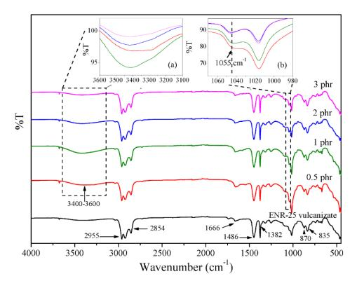
Figure 2. FT-IR spectra of ENR-25 vulcanizate and all rubber composites with varying LCNO contents.
