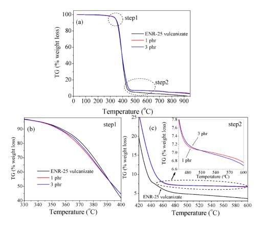
**Figure 1.** TGA curves of (a) ENR-25 vulcanizate and the selected rubber composites with various LCNO contents, the expand scale of temperature degradation of (b) the first step and (c) the second step, respectively.
