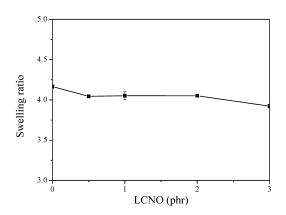
**Figure 4.** Swelling ratio of ENR-25 vulcanizate and the rubber composites with the different addition of LCNO filler.
