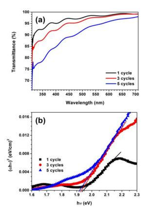
**Figure 4.** (a) Optical transmittance; and (b) optical band gap energy of CuO films prepared on FTO substrate for different cycles.
