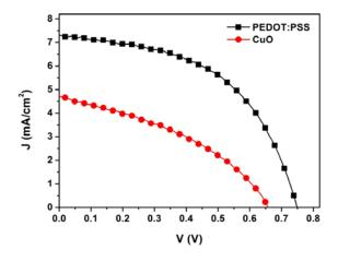
**Figure 6.** Current density - voltage characteristics under standard illumination of p-i-n perovskite solar cell fabricated with PEDOT:PSS and CuO films.
