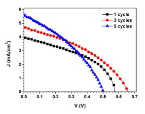
**Figure 5.** Current density versus voltage of p-i-n perovskite solar cell fabricated with CuO films.
