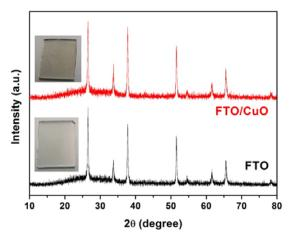
**Figure 3.** XRD patterns of FTO substrate and FTO/CuO films.
