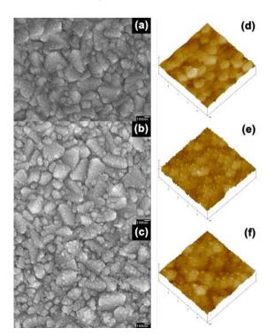
**Figure 1.** SEM images and AFM images of CuO film prepared on FTO substrate with different number of cycles: (a,d) 1, (b,e) 3, and (c,f) 5.
