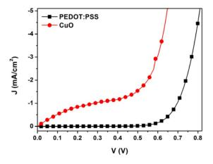
Figure 8. Current density - voltage characteristics measured under dark conditions.
