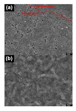
**Figure 7.** Morphology of perovskite films coated onto (a) FTO/CuO and (b) FTO/PEDOT:PSS.
