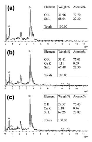
**Figure 2.** Chemical elements of CuO films prepared on FTO substrate with different number of cycles: (a) 1, (b) 3, and (c) 5.
