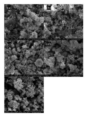
Figure 2. Scanning electron micrographs showing particle morphology of powders prepared by solution
