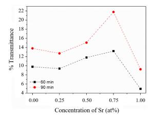
**Figure 4.** Light transmittance of the suspension containing  $Sr_xCa_{(1-x)}TiO_3$ , where x=0, 0.25, 0.5, 0.75 and 1, with the measurements conducted at 60 and 90 min after exposing to UV irradiation.
