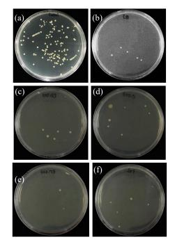
Figure 6. Antibacterial test of powders with compositions: (a) Control-no powder addition, (b) with  $CaTiO_3$  powder, (c) with  $Sr_{0.25}Ca_{0.75}TiO_3$  powder, (d) with  $Sr_{0.5}Ca_{0.5}TiO_3$ powder, (e) with  $Sr_{0.75}Ca_{0.25}TiO_3$  powder, and (f) with  $SrTiO_3$  powder.
