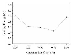
**Figure 3.** Bandgap energy of  $Sr_xCa_{(1-x)}TiO_3$ , where x=0, 0.25, 0.5, 0.75 and 1.
