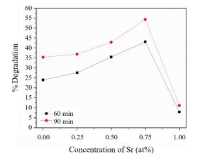
**Figure 5.** Degradation of methylene blue containing  $Sr_xCa_{(1-x)}TiO_3$ , where x=0, 0.25, 0.5, 0.75 and 1 powder, with the measurements conducted at 60 and 90 min.
