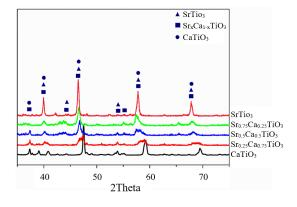
**Figure 1.** X-ray diffraction pattern of  $Sr_xCa_{(1-x)}TiO_3$ , where x=0, 0.25, 0.5, 0.75 and 1 powder synthesized by solution combustion technique.
