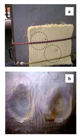
**Figure 4** Testing of 30 layers of aramid fabric with .44 magnum: (a) stop of the bullet in the Kevlar and (b) indentation of the modeling clay at the back of the aramid fabric.
