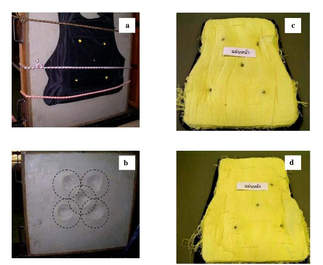
**Figure 6** Testing of bulletproof vest from bullet impact: (a) clamping the vest with modeling clay; (b) indentation of modeling clay after the bullet impact on the vest (front size); (c) bullet blocked in the front size of the vest and (d) bullet blocked in the back size of the vest.
