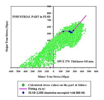
**Figure 12.** Verification of the FLSD criterion uncoupled with Hill48's yield criterion (isotropic condition) with an industrial part made of SPCE 270.
