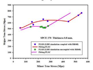
Figure 10. Comparison between the FLSDs calculated by simulations coupled and uncoupled with Hill 48's yield criterion.
