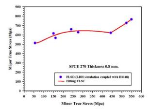
Figure 9. Determined forming limit stress diagram (FLSD) coupled with Hill48's yield criterion (anisotropic condition).
