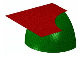
**Figure 6.** A quarter model of punch and specimen used in FEM simulation for the FLSD determination.
