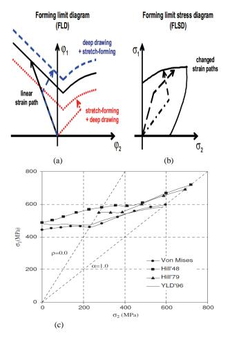
**Figure 1.** (a) Strain based failure criterion FLD <sup>(18, 20)</sup> (b) and stress based failure criterion FLSD <sup>(18, 20)</sup>, and (c) Forming limit stress diagram of a bake-Hardening Steel (BH steel) coupled with different yield criteria<sup>(7)</sup>.
