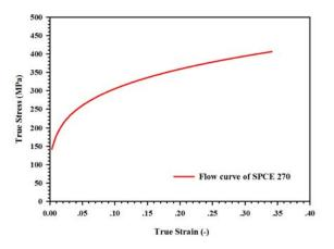
Figure 7. Flow curve of SPCE 270 steel sheet.
