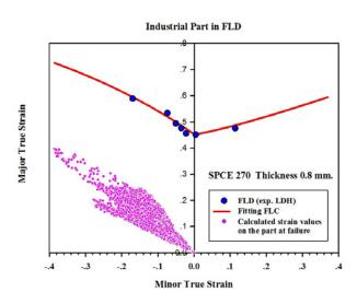
Figure 11. Verification of the FLD criterion with an industrial part made of SPCE 270.
