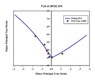
Figure 5. Determined forming limit diagram for SPCE 270 steel sheet.
