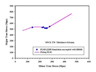
Figure 8. Determined forming limit stress diagram (FLSD) uncoupled with Hill48's yield criterion (isotropic condition).
