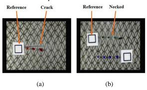
Figure 4. (a) Deformation of circular grids near surface crack. (b) Deformation of circular grids in necked area<sup>(14)</sup>.
