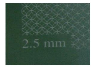
**Figure 3.** Circular Grids were marked onto the surface of blank sheet using electrochemical-etching technique <sup>(14)</sup>.
