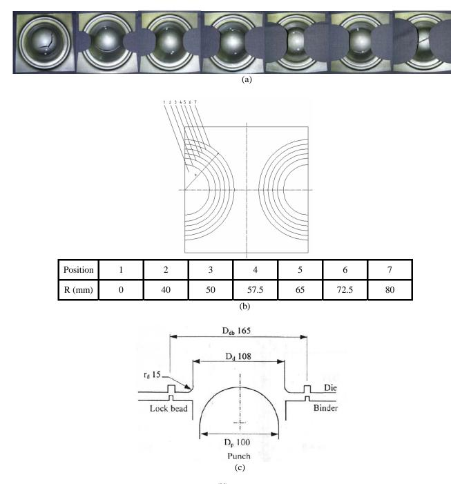
**Figure 2.** Limit dome height test for determining FLD<sup>(14)</sup> (a) A pressed specimen at fracture after LDH test, (b) specimen geometries, and (c) tool drawing of LDH test.
