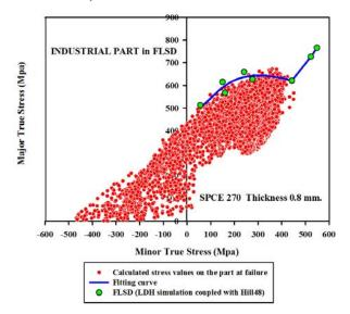
**Figure 13.** Verification of the FLSD criterion coupled with Hill48's yield criterion (anisotropic condition) with an industrial part made of SPCE 270.
