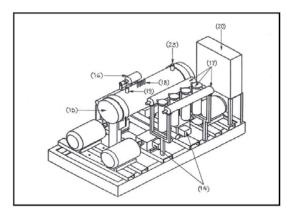
Figure 2. Full Set of High Water Pressured Pump with 280 bar and Flow Rate at 80 liters/min.
