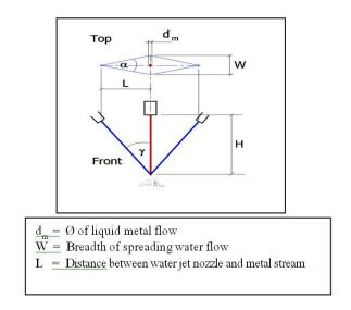
Figure 13. Configuration of main water jet nozzle.
