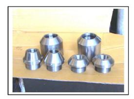
Figure 5. Changeable Cone Nozzles.
