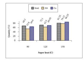
Figure 10. Powder Yield Quantity from Ø5 mm Nozzle.
