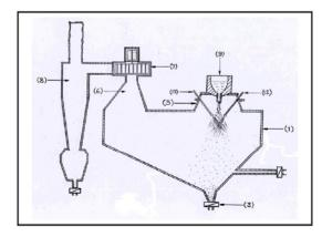
Figure 1. Internal Description of a Water Atomizing Machine.
