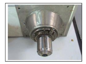
Figure 4. Inverted Cone Shaped Nozzle.
