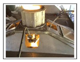
Figure 3. Molten Metal Spraying by V-jet Nozzle.
