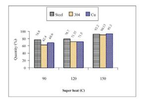
Figure 11. Powder Yield Quantity from Ø6 mm Nozzle.
