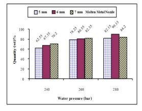
Figure 8. Yield quantity (%wt) of AISI 304 stainless steel powder obtained from 10 kg of raw metal.
