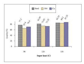
Figure 12. Powder Yield Quantity from Ø7 mm Nozzle.
