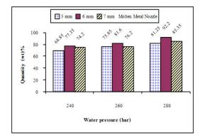
Figure 7. Yield quantity (%wt) of low carbon steel powder obtained from 10 kg of raw metal.
