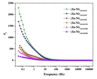
**Figure 5.** Relative permittivity of CMMA (Zn-Ni)<sub>2.0/4.0</sub> coatings with varying number of layers as function of frequency
