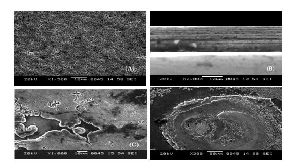
**Figure 8.** SEM image of (Zn-Ni) <sub>2.0/4.0/30</sub> (A), cross-sectional view of (Zn-Ni)<sub>2.0/4.0/30/triangular</sub> (B) and monolayer (Zn-Ni)<sub>3.0</sub> and CMMA (Zn-Ni)<sub>2.0/4.0/6</sub>, after corrosion test [(C) and (D)].
