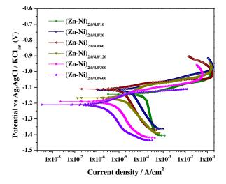
**Figure 2.** Potentiodynamic polarization curves of CMMA (Zn-Ni)<sub>2.0/4.0</sub> coatings with different number of layers.
