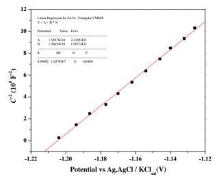
**Figure 4.** Mott- Schottky plot for CMMA (Zn-Ni)<sub>2.0/4.0/600</sub> coating developed at optimal bath conditions.
