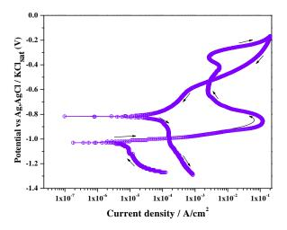
Figure 6. Cyclic polarization curve of CMMA  $(Zn-Ni)_{2.0/4.0/600}$  coating developed at optimal bath condition.
