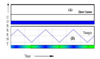
Figure 1. Schematic representation of (A) Monolayer Zn-Ni alloy using constant current, and (B) Composition graded multilayer coating using triangular current pulses, cycling between pre-defined current densities.
