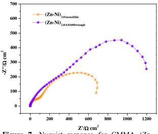
**Figure 7-** Nyquist response for CMMA (Zn-Ni)<sub>2.0/4.0/600/triangular</sub> and monolithic (Zn-Ni)<sub>3.0</sub> coatings of the same thickness.
