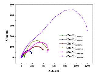
**Figure 3.** Real versus imaginary resistance values of CMMA (Zn-Ni)<sub>2.0/4.0</sub> coatings with different number of layers measured as function of frequency.
