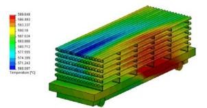
**Figure 5.** Temperature gradient of the stacking of billets during Homogenization analyzed by COSMOSFloWorks<sup>TM</sup>.
