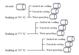
Figure 2. Conditions of specimens, i.e. as-cast and homogenizing at 585°C, 575°C and 565°C cooled by different methods.
