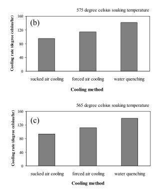
**Figure 4.** A summary of cooling rates of soaked billet at (a) 585°C, (b) 575°C and (c) 565°C with sucked air cooling, forced air cooling, and water quenching.
