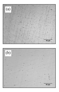
Figure 6. Microstructure of (a) as-cast billet contained β-AlFeSi and Mg2Si and (b) homogenized billet contained α-Al(FeMn)Si. Mg2Si precipitates were dissolved.
