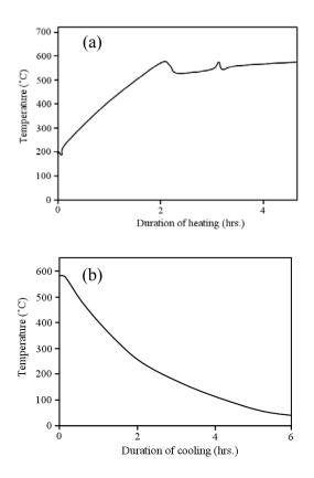
Figure 3. The relationship between temperature of aluminum billets and time during (a) homogenizing at 585°C and (b) cooling.
